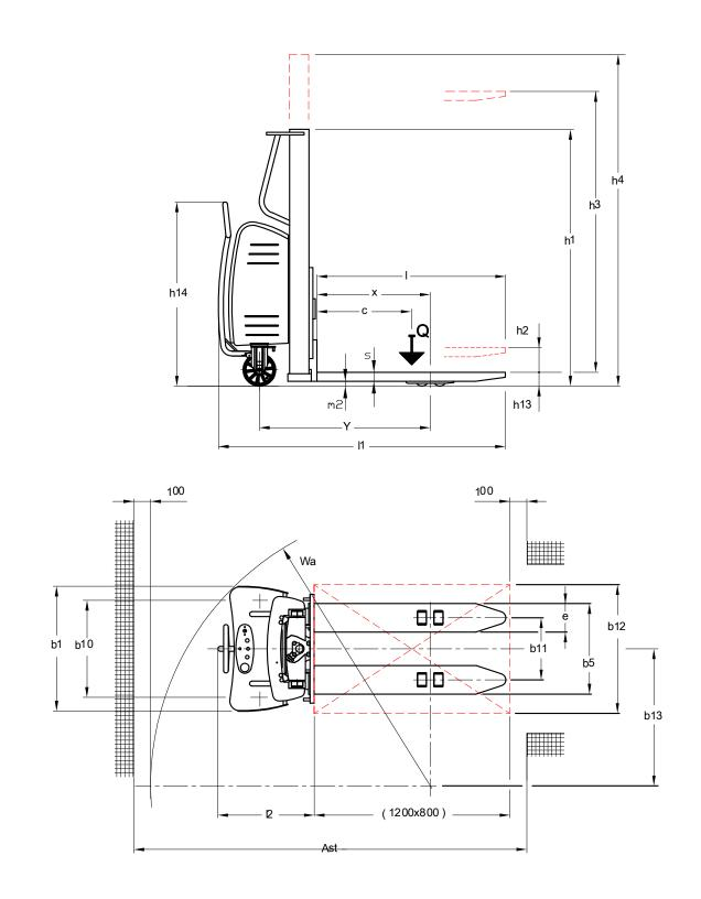
VDI 2198 - Four wheel Forklift Truck top view, reduced load width -  $b12/2 \le b13$
